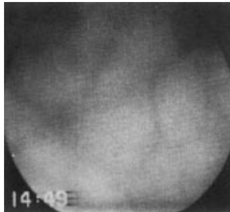
Figure 12. Network pattern observed at the surface of molten silicon (Yamagishi & Fusegawa 1990).
